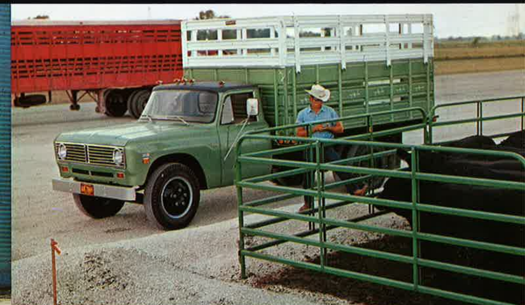
MODEL 1510 , shown above with combination stock and grain rack—the ideal body for farmers. Wheelbases are 132 inches for 9-foot stake or platform bodies, or 156 inches for 12-foot stake, platform, dump or van bodies. GVW ranges up to 15,000 pounds.
