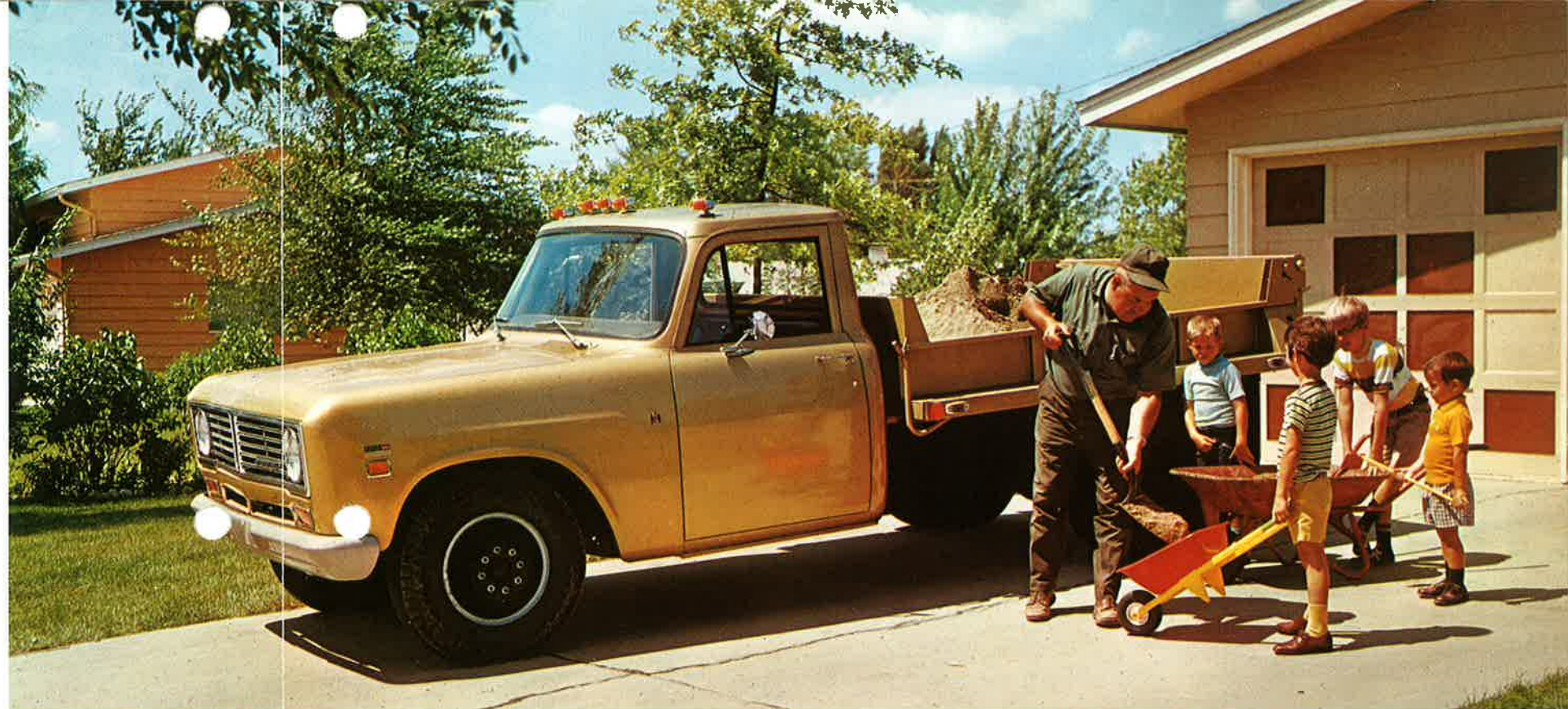
MODEL 1310 , shown above with dump bed which is ideal for contractors, landscapers, cemeteries, municipalities, and many other uses. Wheelbases are 131 inches for 8-foot regular or Bonus-Load pickup bodies, 134 inches for 9-foot regular pickup, dump, stake or platform bodies, 156 inches for 12-foot stake, dump, platform or van bodies. GVW ranges up to 10,000 pounds.
