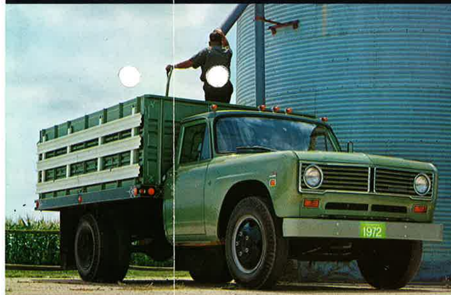
MODEL 1510 , shown above with combination stock and grain rack—the ideal body for farmers. Wheelbases are 132 inches for 9-foot stake or platform bodies, or 156 inches for 12-foot stake, platform, dump or van bodies. GVW ranges up to 15,000 pounds.
